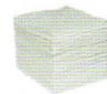
Oil-Only Sonic Bonded Pads Composition: Polypropylene Dimensions: 19"L x 15"W Absorbency: 1.1 liter
